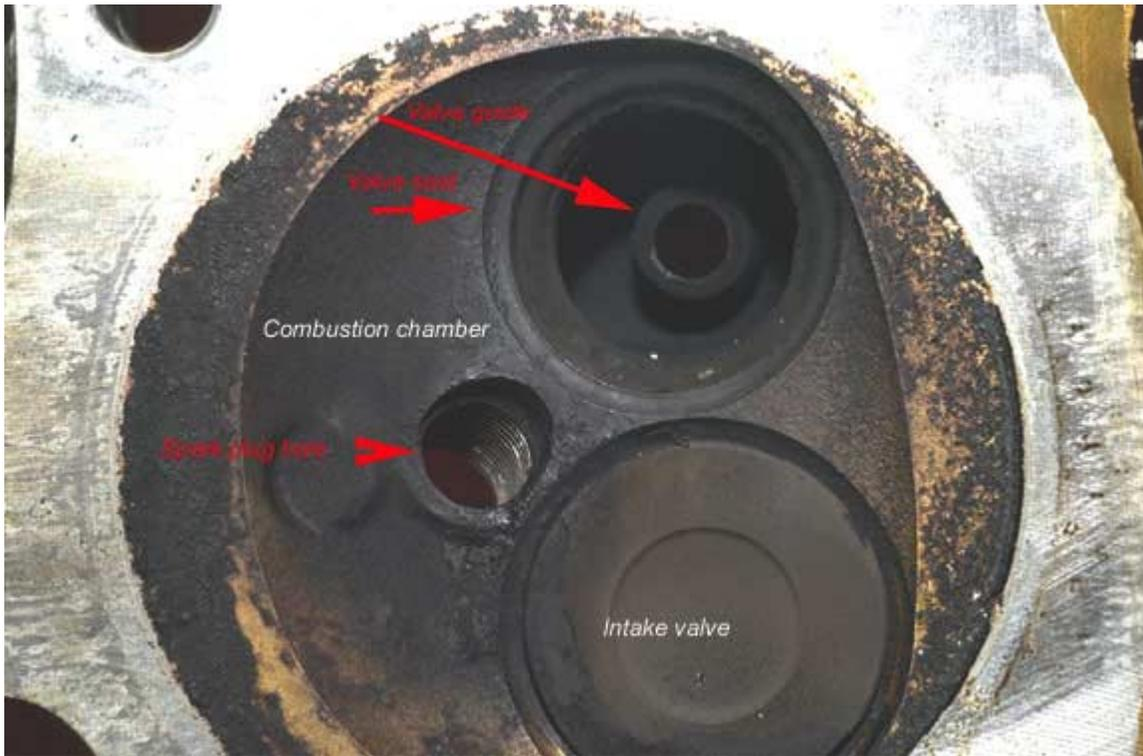
Having taken the head off, we can remove a valve spring and pull one of the sticky valves. Here's what a sticky valve looks like up close
