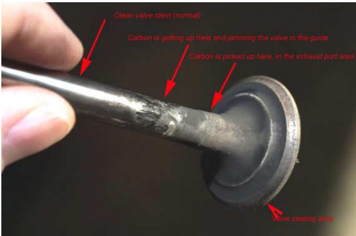
You can see what is happening. The lower part of the valve (on the right) picks up a coating of carbon from the hot exhaust gases heading out the port (The exhaust port is the passage in the head leading to the exhaust system. The intake port leads from the intake valve to the intake manifold). This carbon works its way up the valve. The clearance between the valve and the valve guide is tight – perhaps one
