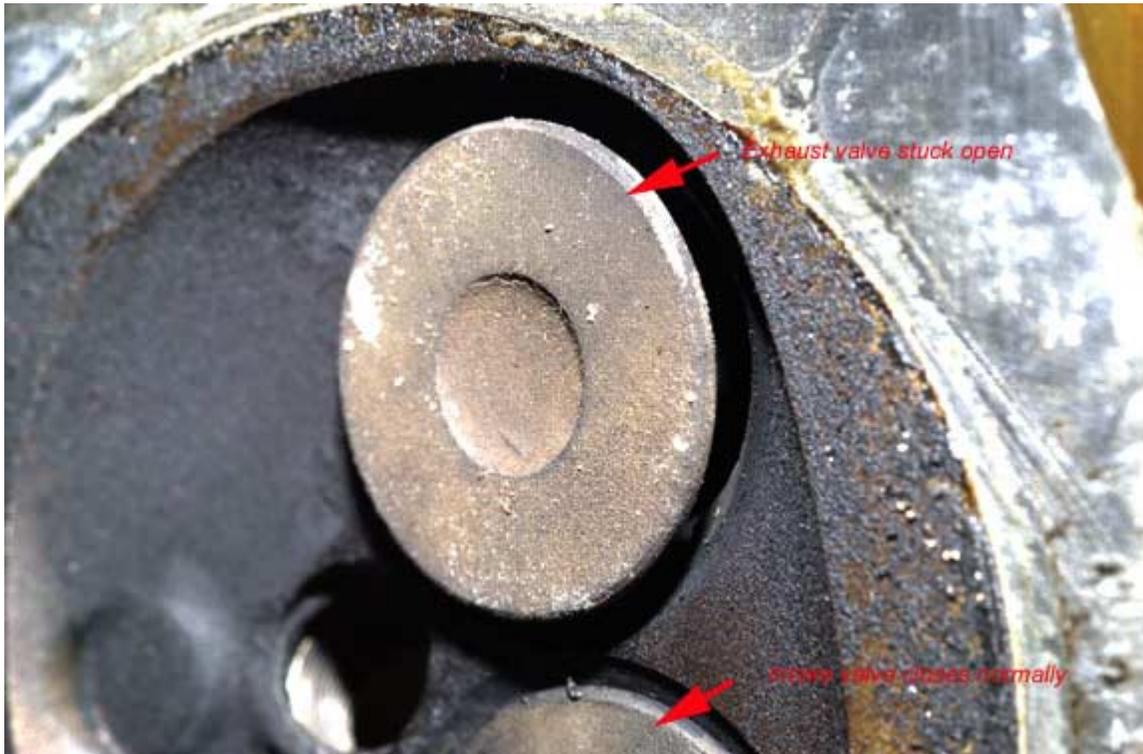
Here we've removed the valve, and the carbon buildup on the seat is quite evident. With carbon buildup like this on the seat, it's a safe bet this engine was down on power all the time. Once we've fixed it it's owner will surely see an increase in performance. The hole in the center of the port is the valve guide. The guide, seat, and head look like areas on one piece of metal but they are actually three distinct parts.
